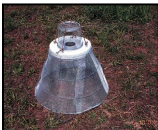
Fig. 2. Previous fire ant alate trap with inverted wire basket and screening that funnels alates initiating flights into a pan filled with collecting fluid.
