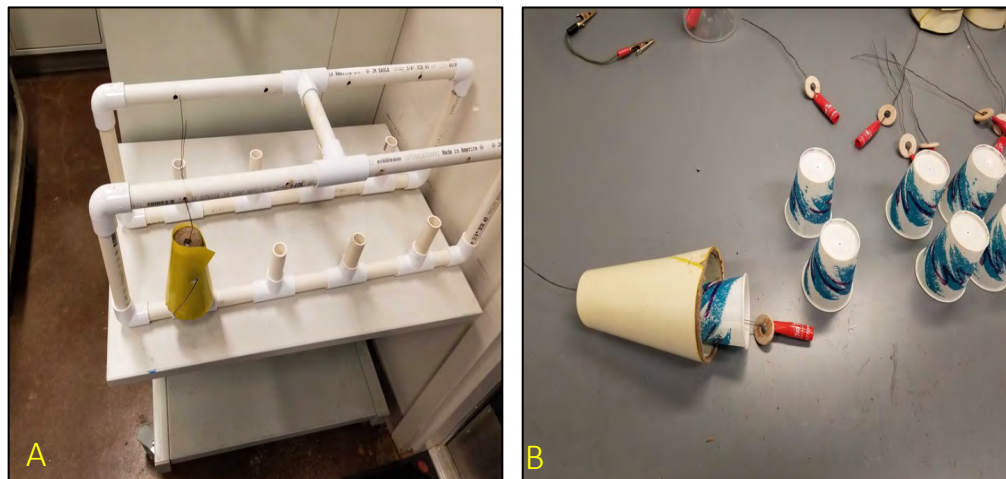
Figure 3. Trap transport and assembly. The adhesive on the sticky paper created several challenges in the field. (A) A PVC rack was constructed to help move traps between the lab and field sites. (B) Dixie cups were used to prevent the contact between the user's skin and the sticky paper during trap assembly.
