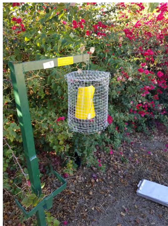
Figure 4. Trap cage. A mesh cage was constructed to prevent local wild life from coming into contact with the sticky traps.
