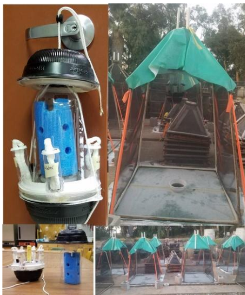
Figure 1. QM-ATSB design (left) and UC Riverside field deployment (right) of fungal and chemical control agents.
