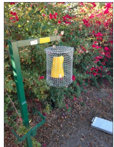
Sticky trap used in study. The mesh cage protects the sticky trap.
