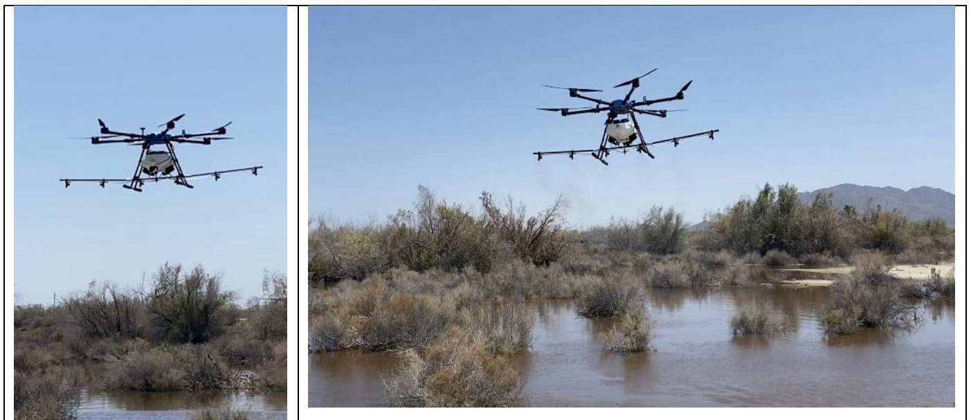
Leading Edge PV35X UAS set with liquid application equipment, performing a treatment along the Salton Sea Westshore.
