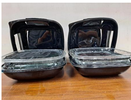
Figure 2. Bait dispensers with sealed reservoirs (maximum volume = 1700 mL) accessible by a hollowed-out mesh feeding surface used in spring 2021 (right) compared to the previous design (left).
