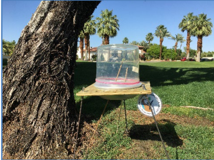
Fig. 4. Dec.2021 trap design with a plywood base that provided more secure attachment points for the legs.
